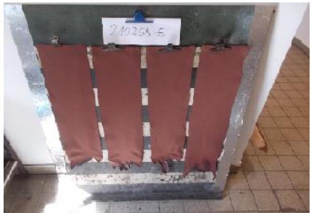
2.3 Normal flammability test according to DIN 4102-1
