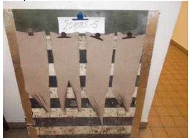
2.3 Normal flammability test according to DIN 4102-1
