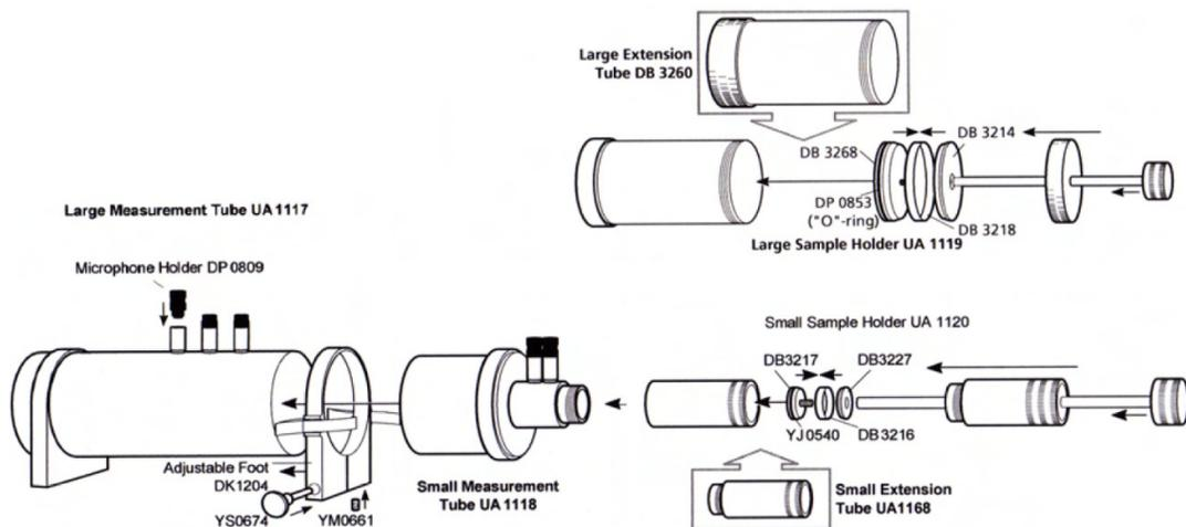
Figure 2: Breakdown of Impedance Tube components<sup>1</sup>
