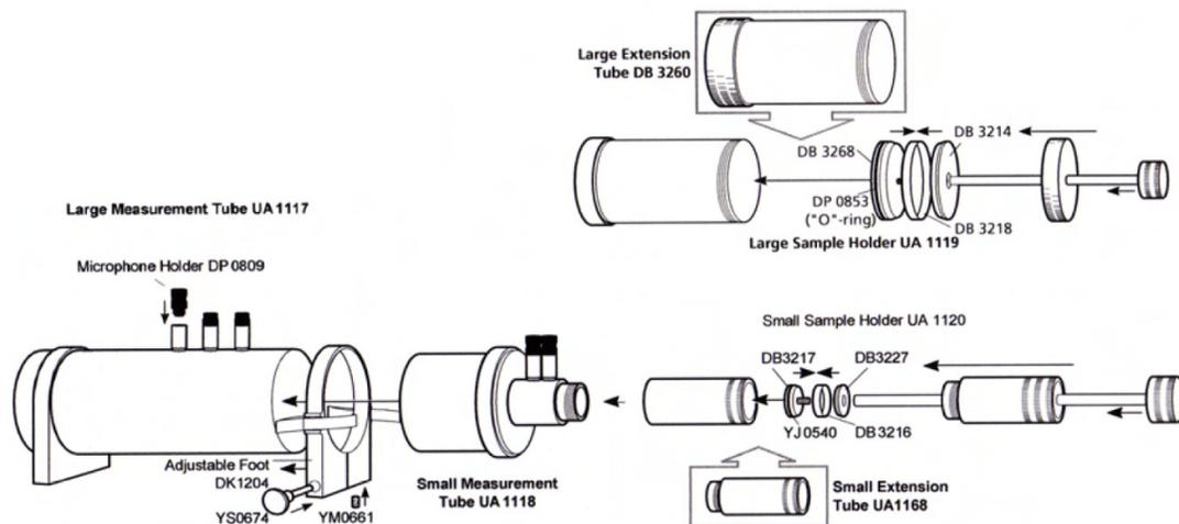
Figure 2: Breakdown of Impedance Tube components<sup>1</sup>
