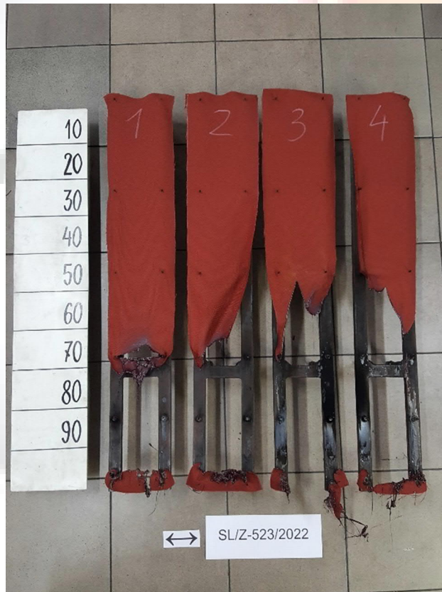
Figure 2. Appearance of the sample 1 after the test - cross direction
