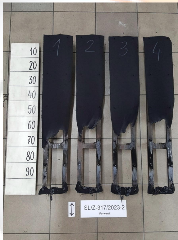
Figure 4. Appearance of the sample 3 after the test – Forward – length direction
