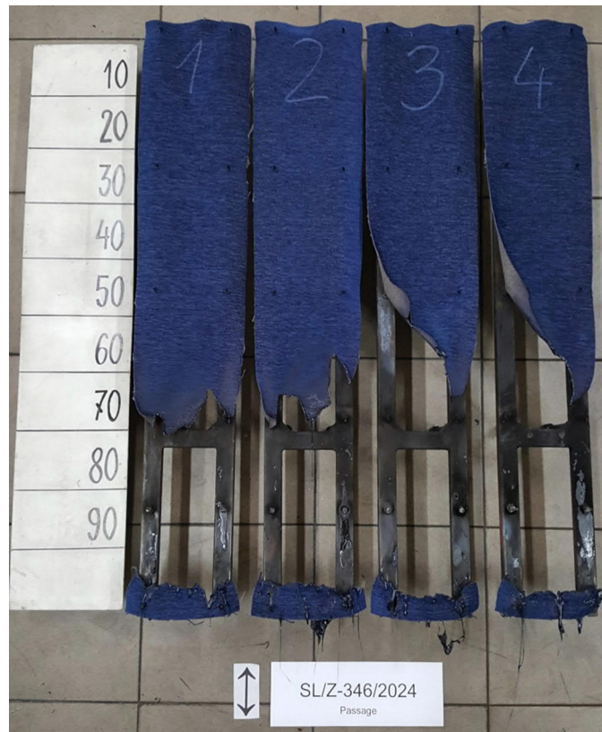
Figure 5. Appearance of the specimens 4 after the test – dark blue color
