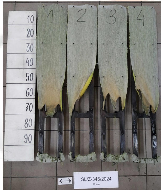
Figure 2. Appearance of the specimens 1 after the test – white-light green color
