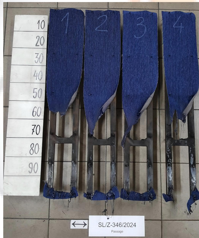
Figure 4. Appearance of the specimens 3 after the test – dark blue color
