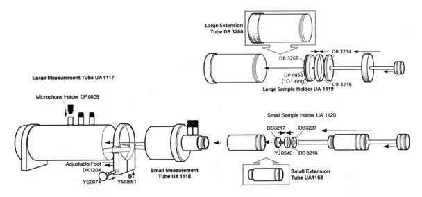
Figure 1: Brüel and Kjær Type 4206 Impedance Tube Components
