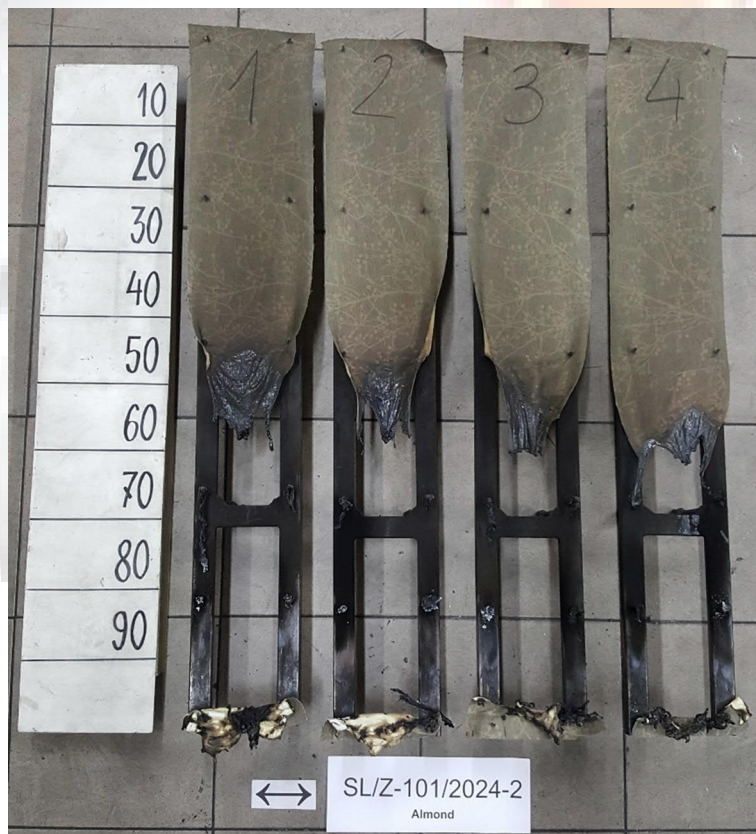
Figure 4. Appearance of the sample 3 after the test – Almond/212275-15 – cross direction
