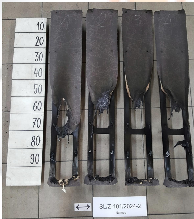
Figure 2. Appearance of the sample 1 after the test – Nutmeg/212275-14 – cross direction
