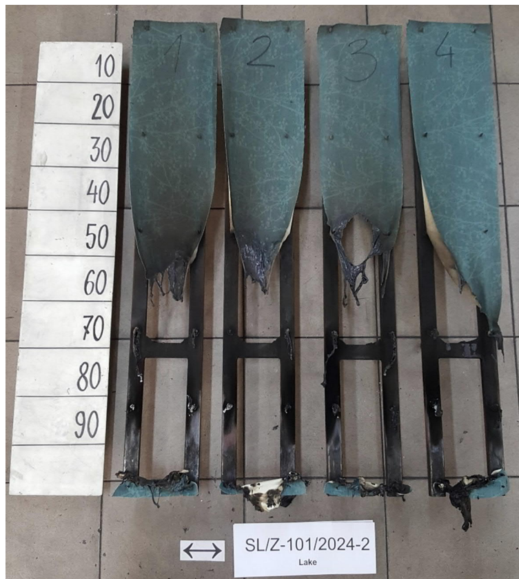
Figure 5. Appearance of the sample 4 after the test – Lake/212275-16 – cross direction
