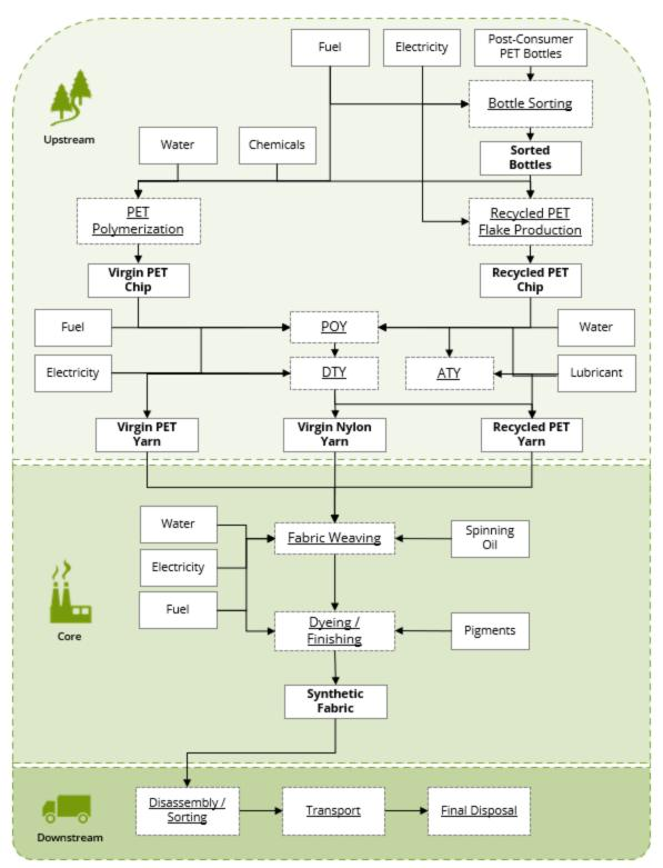
**Figure 2.** Flow Diagram representing the major processes in each life stage included within the life cycle of the synthetic textile products. Underlined text in dashed line boxes represent processes, while plain text-solid line boxes represent inputs, and bold text boxes represent key outputs.
