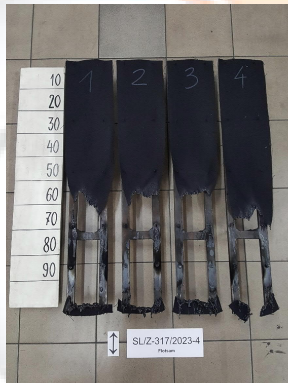
Figure 4. Appearance of the sample 3 after the test – Flotsam – length direction
