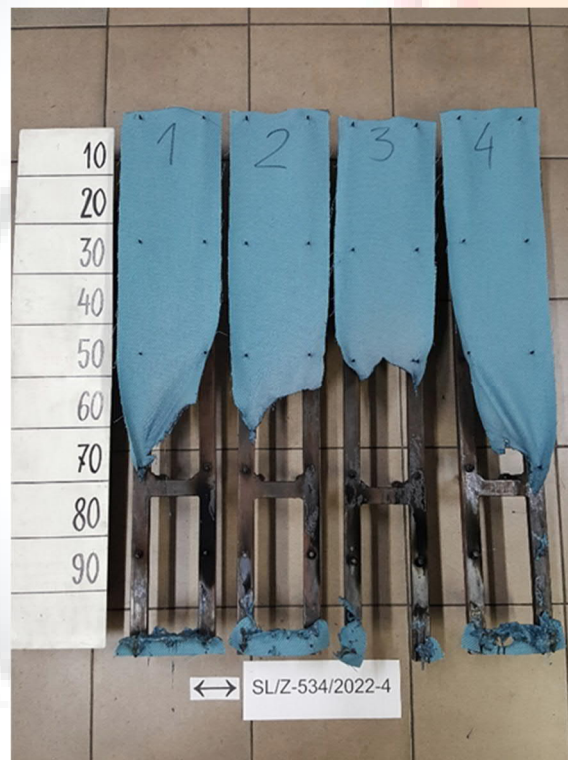
Figure 2. Appearance of the sample 1 after the test – HOOC02 – cross direction
