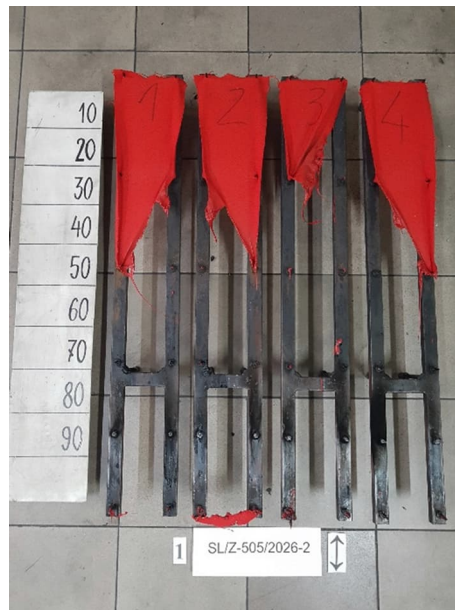
Figure 5. Appearance of the sample 4 after the test – “Medium Colour: Redstone - Batch: 586326”, length direction
