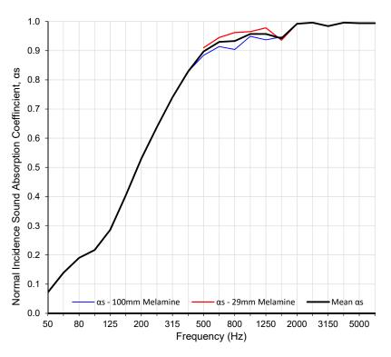
Figure 3: Normal incidence sound absorption coefficient  $\alpha_{\rm S}$  of the melamine foam.
