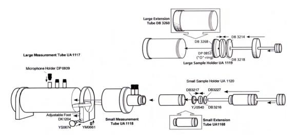
Figure 2: Breakdown of Impedance Tube components<sup>1</sup>
