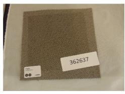
REQUEST: Colour fastness to chlorinated water using a 1.3% chlorine solution
