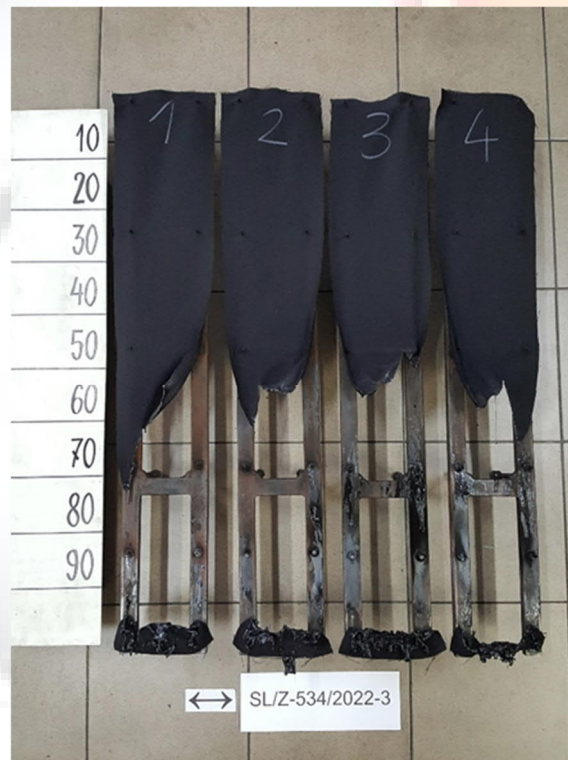
Figure 2. Appearance of the sample 1 after the test – HQUE01 – cross direction
